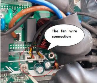
Step 4. If step 1-3 have been well checked and the fan still not work, replace the fan (need same model)
